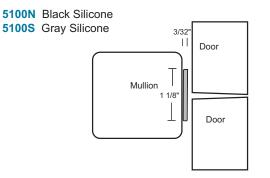
Closed cell silicone sponge strip 1-1/8" wide x 3/32" thick with an adhesive strip for mounting directly to the face of the mullion that doors close against.
